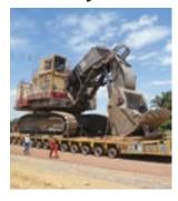
ransportes Montejo has recently transported an 800-ton (727.7-tonne) PC 8000 hydraulic excavator using its Goldhofer PST/SL modular transporter.
